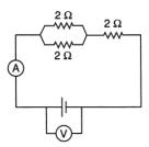
(b) (2 points) Ammeters, wires, and power supplies are assumed to have zero internal resistance as they have no resistance indicated in the circuit diagram. If there were any resistance, unaccounted losses of voltage would occur in our circuit. When
