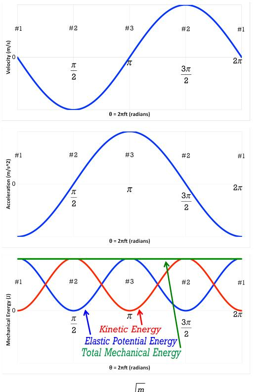
The period of a mass-spring system:  $T_s = 2\pi \sqrt{\frac{m}{k}}$  Is independent of amplitude and acceleration due to gravity. The period of a pendulum:  $T_p = 2\pi \sqrt{\frac{L}{g}}$  Is independent of amplitude and mass.
